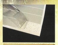
1.) Carefuly "weed" out excess masking film.Lift the mask on one of it's edges. The spaces between the discs should still adhere on the carrier. Remove small remains.
