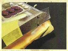
2.) Cut film to length as desired.Cut spaces for details in case.Place some masking tape on uncovered areas to avoid overspray. Make sure the mask has a good contact to surface.
